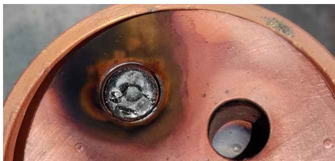
Figure 22: \text{UO}_2 pellet post-arc with shiny spots and puffed surface
