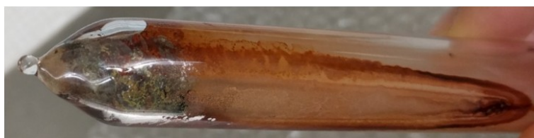
Figure 8: Large batch ampoule after Ramp B. Air sensitive red powder and recrystallized I_2
