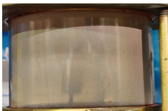
Figure 20: Chamber post-arc. The glass is covered with a red deposit as well as with small black crystals, which seem to confirm the sublimation and deposition of \text{I}_2 .
