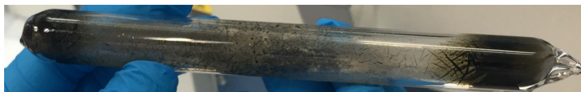
Figure 16: Big batch ampoule showing black dendrites on both ends, dark green deposits, and black bulk at the center
