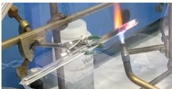
Figure 13: Quartz tube with \text{Dy}_{(m)} and \text{I}_{2(s)} heated directly by flame torch. The heat triggers the reaction which produces the bright glow at the right side of the tube.
