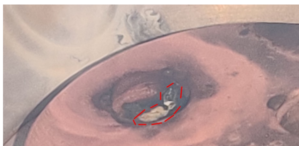
Figure 23: Post-arc UI_3 fragment. The red dotted circle outlines a shiny grey element which might be metal.
