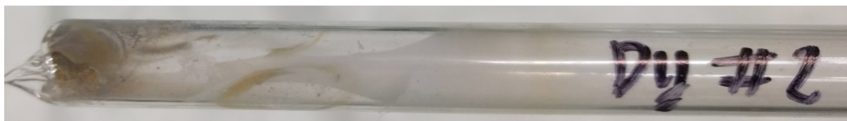
Figure 14: Quartz tube after flame treatment. Metallic bulk with purple shades on the left, white-pink layer deposit on the right.
