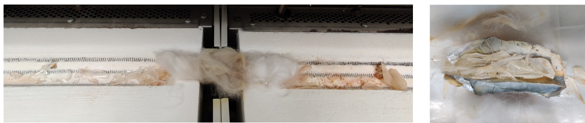
Figure 11: Burst out ampoule in furnace and inside insulation layer
