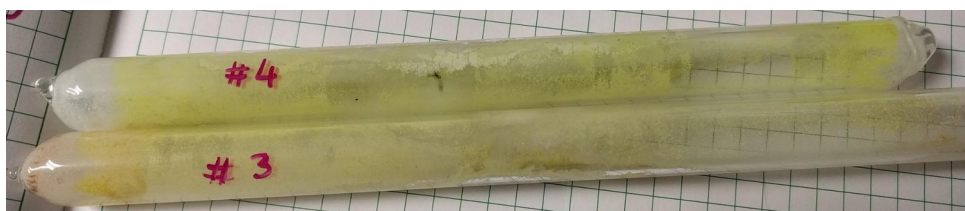
Figure 7: Large batch ampoules after Ramp A. Yellow-lime crystals and white deposits.
